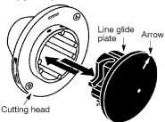
NOTE: Line glide plate must be reinstalled in cutting head before inserting
